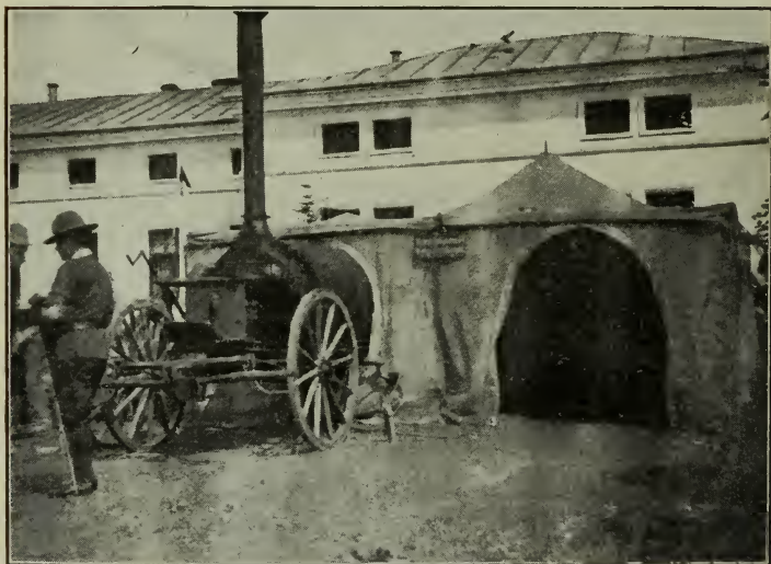
FIG. 35.—Wheeled field oven (Austrian) with tent.
